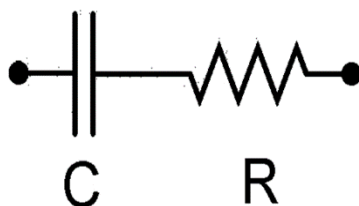
Figure 3.3 Virtual equivalent electronic circuit of a resistor and capacitor in series used for theoretical calculations
